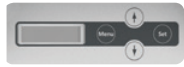
Front control panel with 4 keys, a 2-line LCD display and a status indicator
